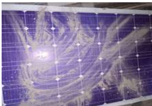
Figure. 1(a) Dust accumulation on the surface of a solar panel
