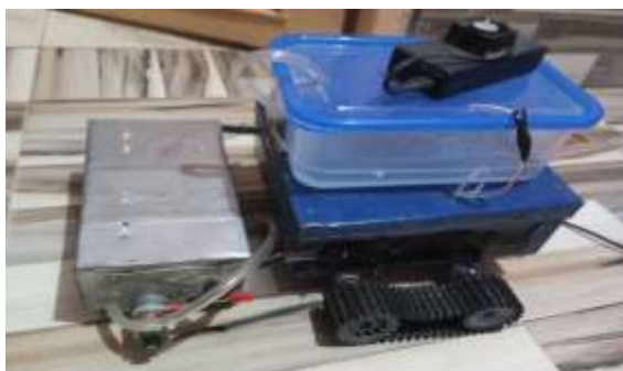
Figure. 1(c) Fig. 3. Prototype solar panel cleaning robot.
